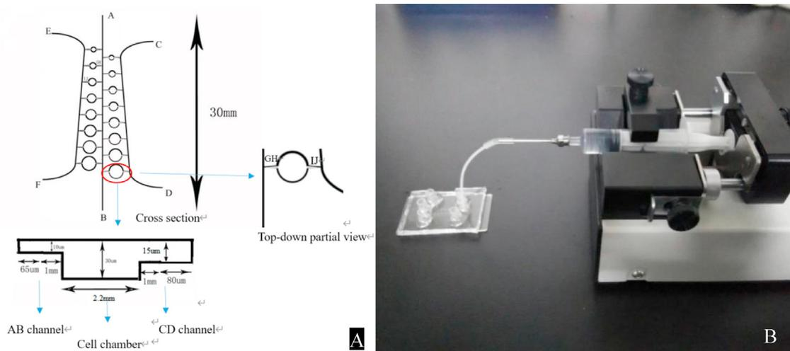
**Fig. 1.** Schematic diagram of chip mask structure. A) Schematic diagram of chip structure; B) Cross-sectional schematic view of the chip channel; C) Image of the fabricated chip.
